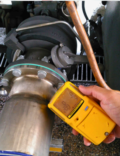
Vapour Testing at Coupler Connection on Site
